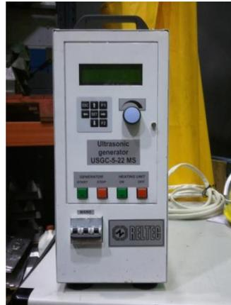
**Figure 4.4.** Ultrasonic controller
