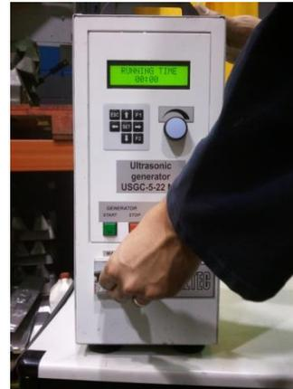
**Figure 4.5.** Turning on the main MCB
