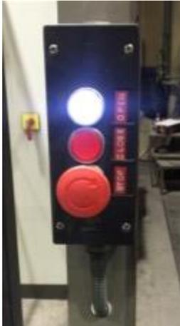
**Figure 5.3.** Keypad of security furnace
