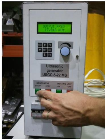
**Figure 4.14.** Turning on the generator
