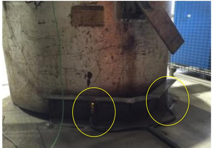
**Figure 5.2.** Activated sensors indicate correct position
